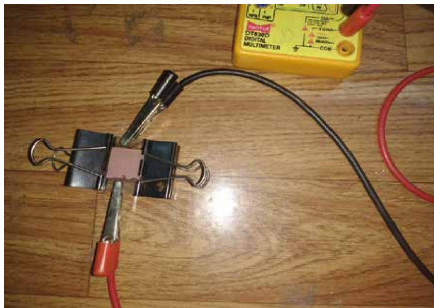
Figure 6: Circuit employed in a DSSC
