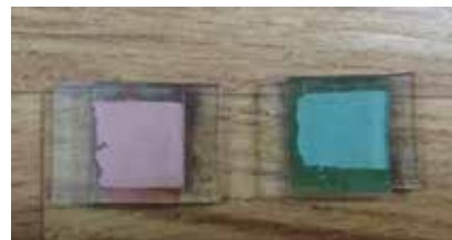
Figure 2: Dye adsorbed on \text{TiO}_2 paste
